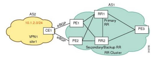
In the following configuration example based on the figure above, RR2 is configured with an additional path, which is a backup path.
