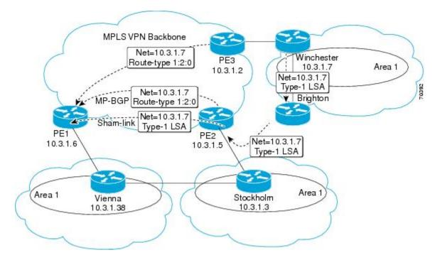
Because the sham-link is seen as an intra-area link between PE routers, an OSPF adjacency is created and database exchange (for the particular OSPF process) occurs across the link. The PE router can then flood LSAs between sites from across the MPLS VPN backbone. As a result, the desired intra-area connectivity is created.
