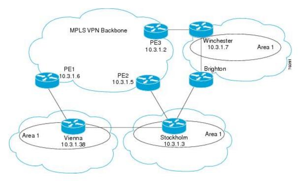
For example, the figure above shows three client sites, each with backdoor links. Because each site runs OSPF within the same Area 1 configuration, all routing between the three sites follows the intraarea path across the backdoor links, rather than over the MPLS VPN backbone.
