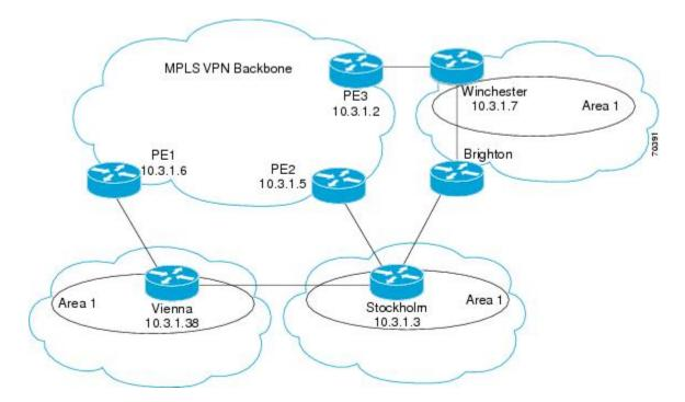
For example, the figure above shows three client sites, each with backdoor links. Because each site runs OSPF within the same Area 1 configuration, all routing between the three sites follows the intraarea path across the backdoor links, rather than over the MPLS VPN backbone.
