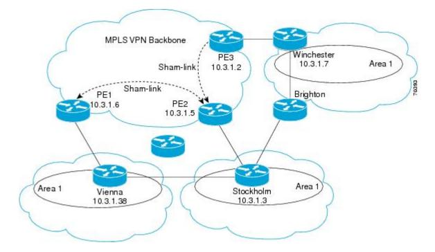
The following example shows the forwarding that occurs between sites from the standpoint of how PE-1 views the 10.3.1.7/32 prefix, the loopback1 interface of the Winchester CE router in the figure above.
