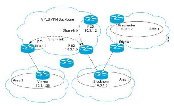
The following example shows the forwarding that occurs between sites from the standpoint of how PE-1 views the 10.3.1.7/32 prefix, the loopback1 interface of the Winchester CE router in the figure above.
