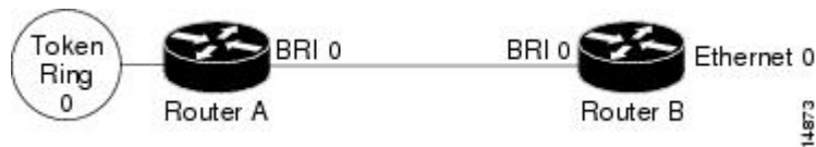
Figure 9: OSPF over On-Demand Circuit
