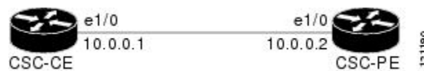
Figure 25: Configuration for Peering with Directly Connected Interfaces Between CSC-PE and CSC-CE Routers
