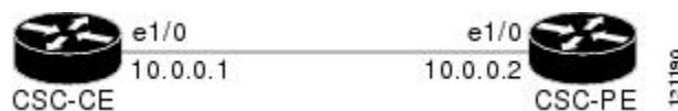
Figure 22: Configuration for Peering with Directly Connected Interfaces Between CSC-PE and CSC-CE Routers
