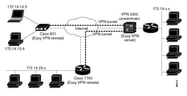
Figure 3: Cisco Easy VPN Network Extension Connection
