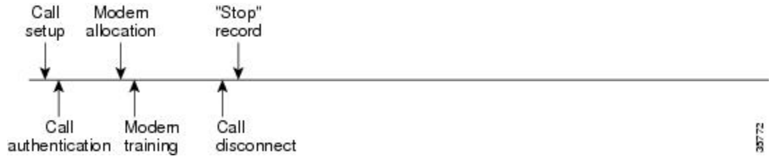
Figure 12: Modem Dial-In Call Setup Sequence With Call Disconnect Occurring Before User Authentication and With Resource Failure Stop Accounting Enabled
