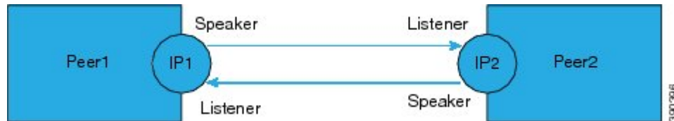
Figure 1: Bidirectional SXP Connection
