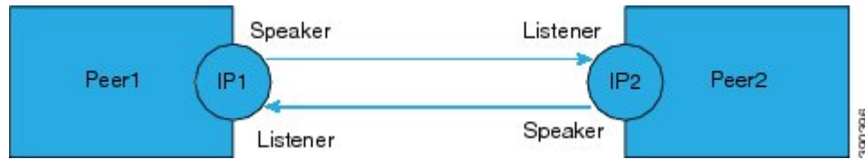
Figure 6: Bidirectional SXP Connection
