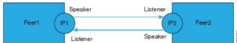
Figure 1: Bidirectional SXP Connection
