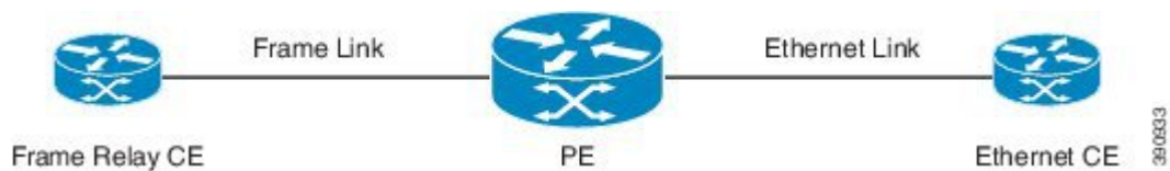
Figure 4: Frame Relay-Ethernet Local Switching Topology
