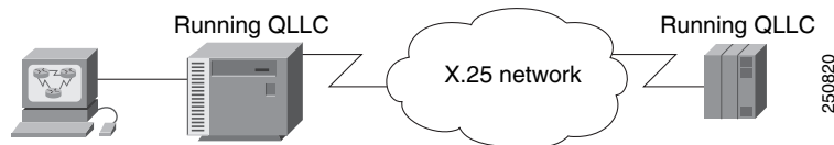
Figure 9 SNA Devices Running QLLC
