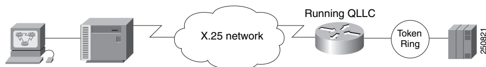
Figure 10 Router Running QLLC Conversion Feature
