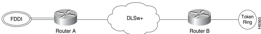
Figure 10 DLSw+ Translation Between FDDI and Token Ring
