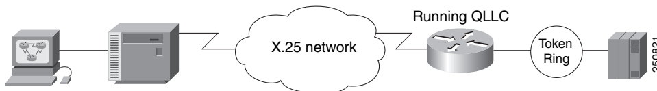
Figure 4 Router Running QLLC Conversion Feature
