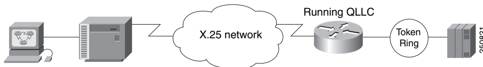
Figure 4 Router Running QLLC Conversion Feature
