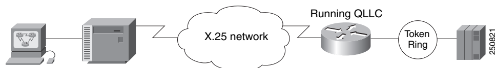
Figure 10 Router Running QLLC Conversion Feature
