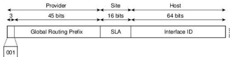
Addresses with a prefix of 2000::/3 (001) through E000::/3 (111) are required to have 64-bit interface identifiers in the extended universal identifier (EUI)-64 format. The Internet Assigned Numbers Authority (IANA) allocates the IPv6 address space in the range of 2000::/16 to regional registries.
