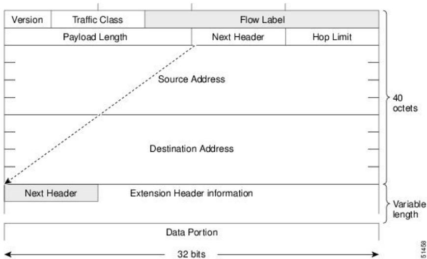
This table lists the fields in the basic IPv6 packet header.
