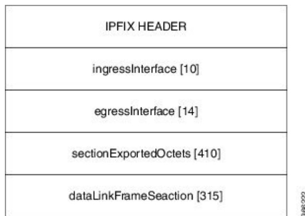
Figure 1: IPFIX 315 Export Packet Format
