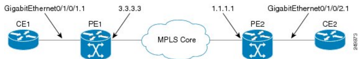
Figure 8: VPWS with BGP autodiscovery and BGP signaling
