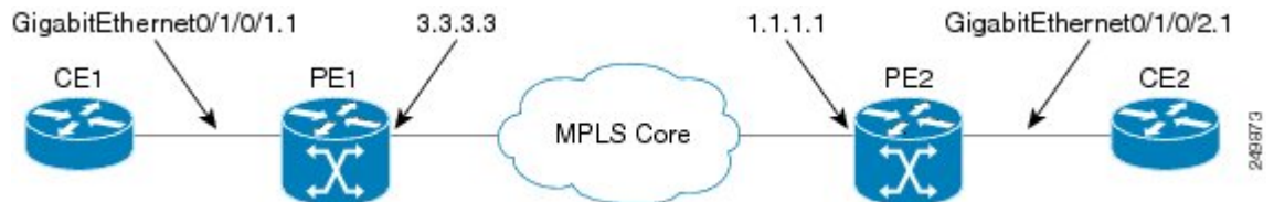
Figure 8: VPLS with BGP autodiscovery and BGP signaling
