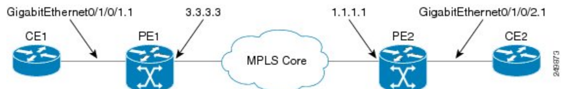
Figure 11: VPLS with BGP autodiscovery and BGP signaling
