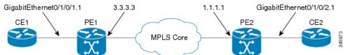
Figure 11: VPLS with BGP autodiscovery and BGP signaling
