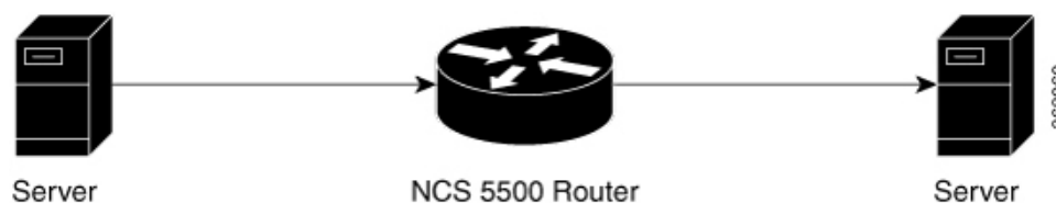
Figure 15: Topology for ERSPAN Egress Rate Limit
