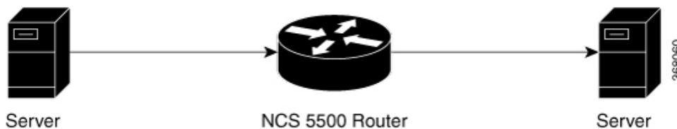
Figure 12: Topology for ERSPAN Egress Rate Limit
