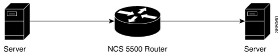
Figure 2: Topology for ERSPAN Egress Rate Limit
