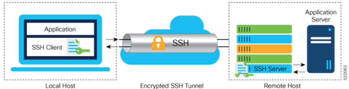
Figure 5: SSH Port Forwarding
