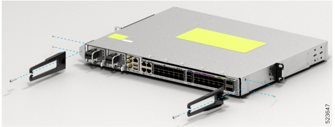
Figure 15: Installing Cable Management and 19 inch Rack-Mount Brackets in the Rear
