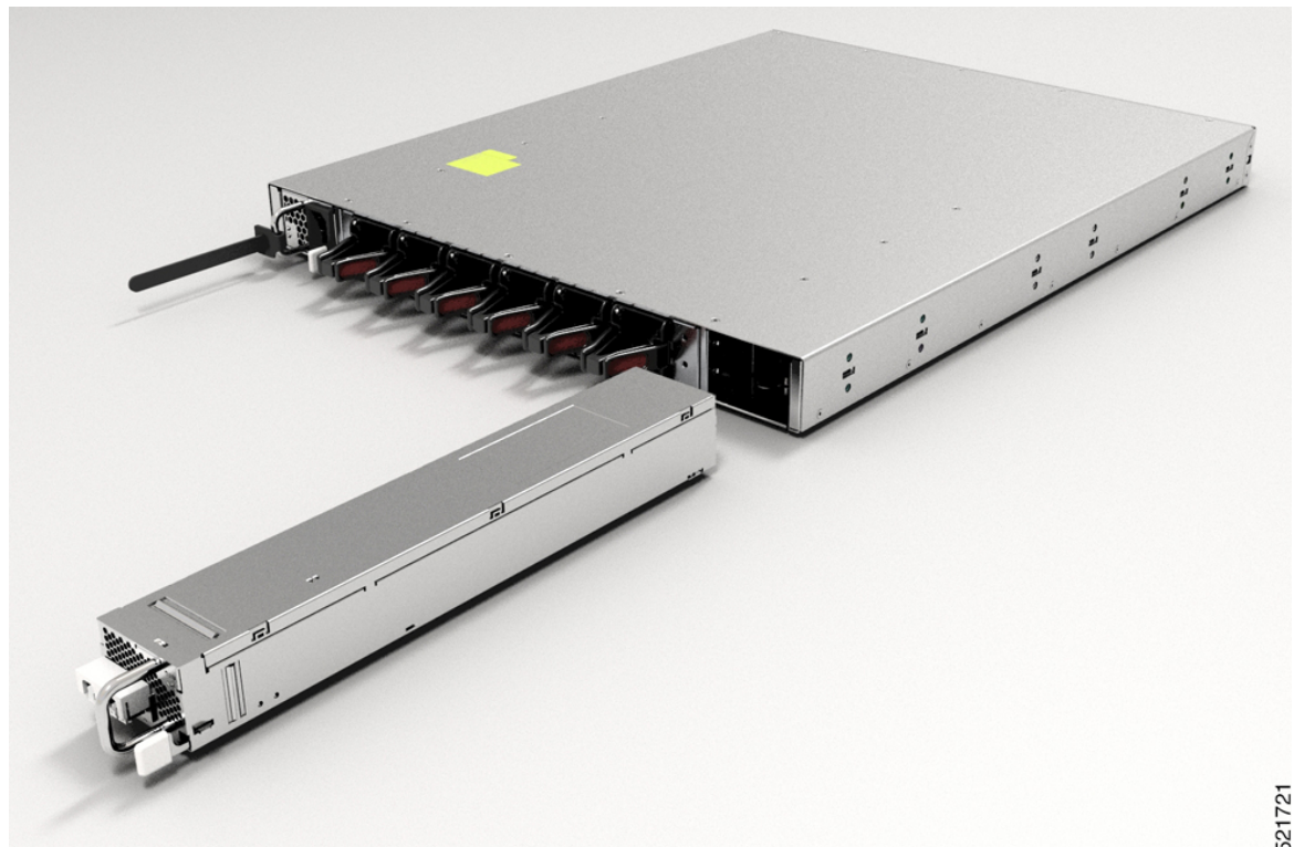
Figure 51: Install DC Power Supply Module for N540-FH-AGG-SYS
