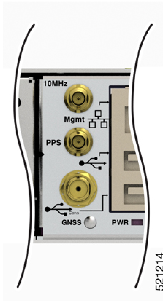
Figure 27: Installing the GNSS Module in the RSP
