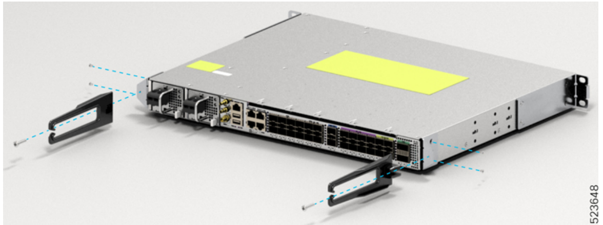
Figure 15: Installing Cable Management and 19 inch Rack-Mount Brackets in the Rear
