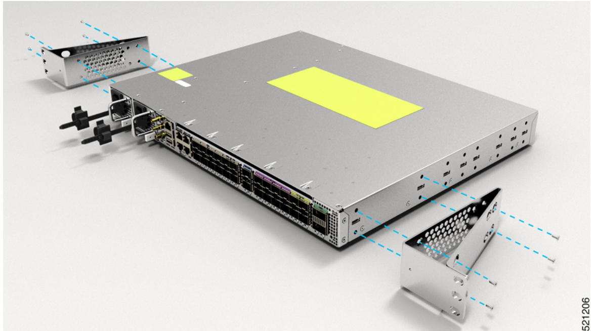
Figure 17: Installing Cable Management and 23 inch Rack-Mount Brackets in the Middle
