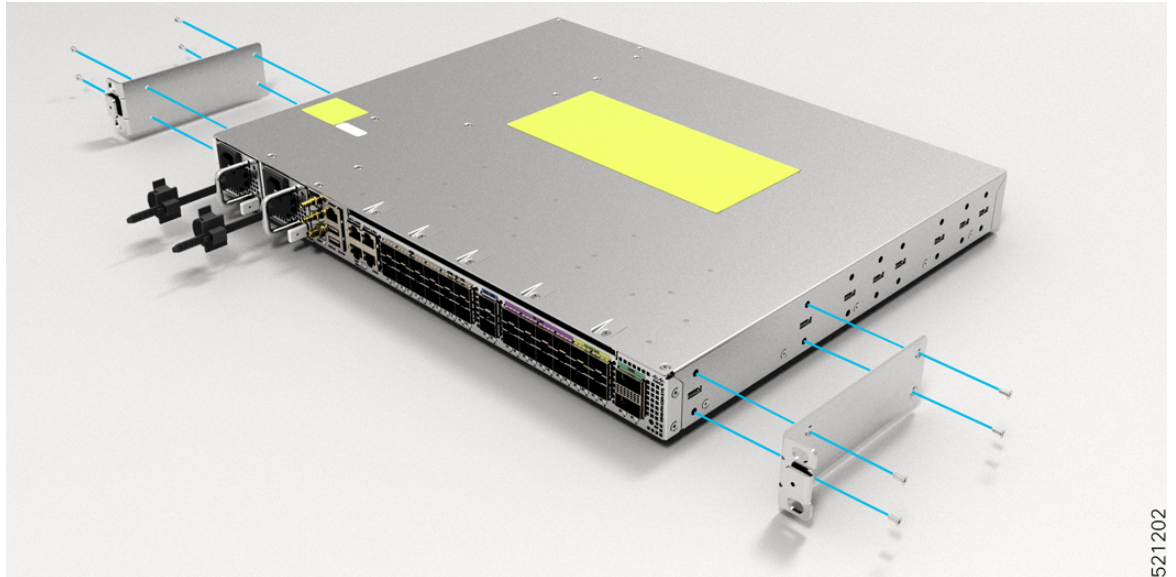
Figure 5: Installing Cable Management and 19 inch Rack-Mount Brackets in the Front
