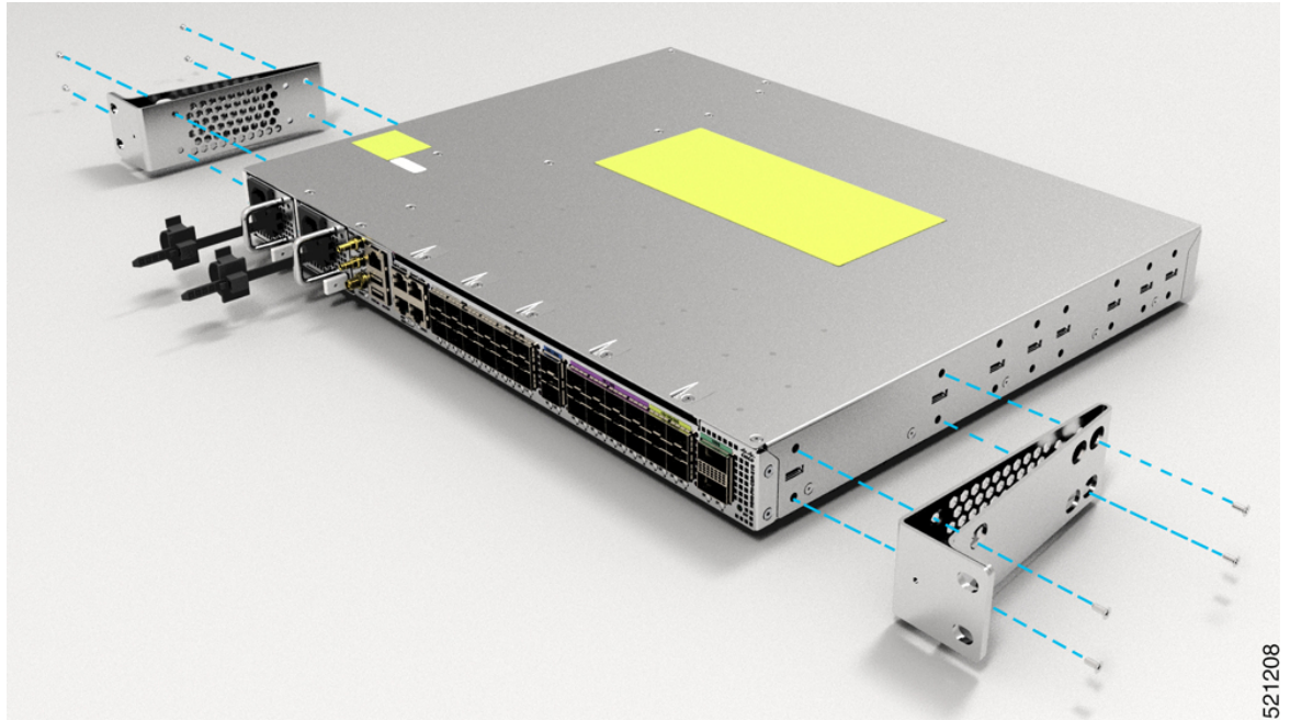
Figure 11: Installing Cable Management and ETSI Rack-Mount Brackets in the Middle
