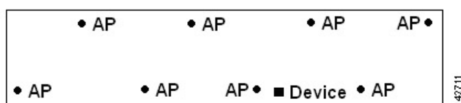
Figure 4: Improved Location Accuracy by Staggering Around Perimeter
