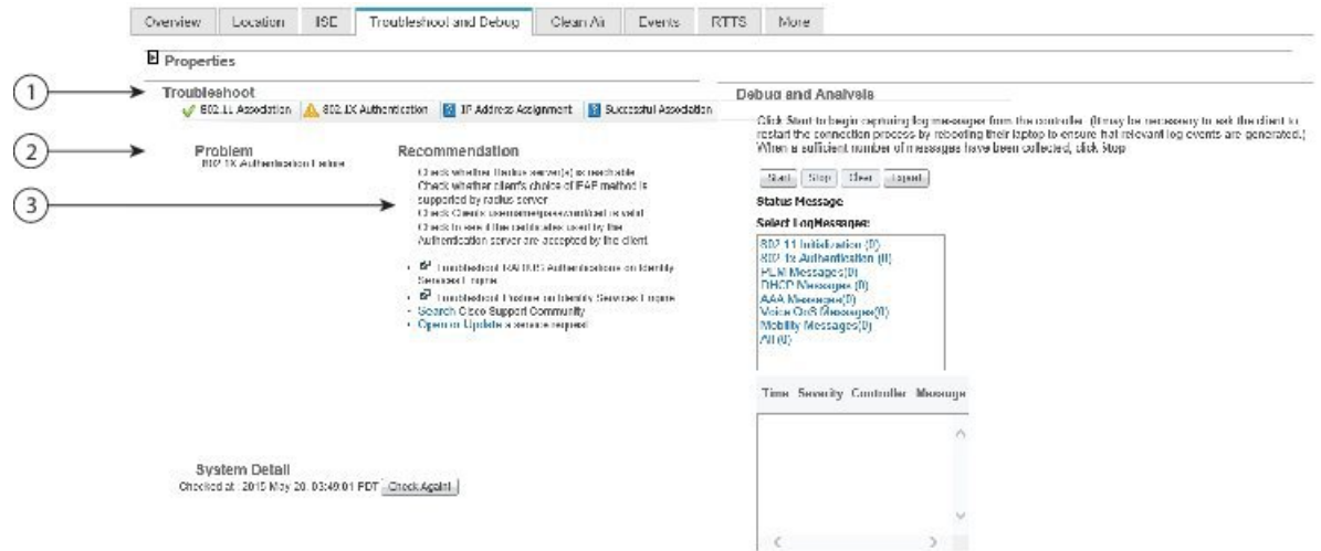
Figure 7: Client Troubleshooting page for Unsuccessful Wireless Client
