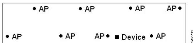
Figure 5: Improved Location Accuracy by Staggering Around Perimeter
