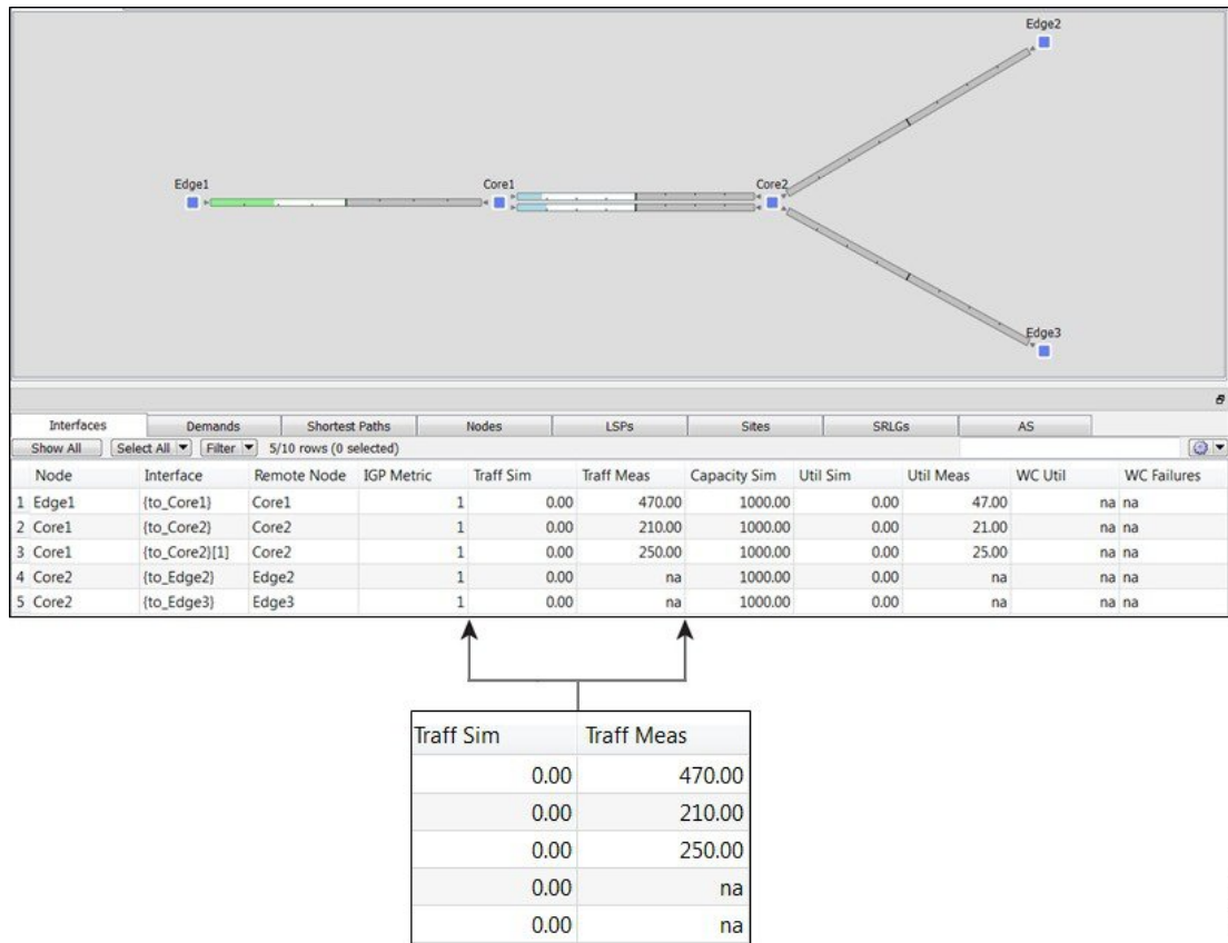
Figure 17: Measured Traffic View and Interfaces Associated with the Demands
