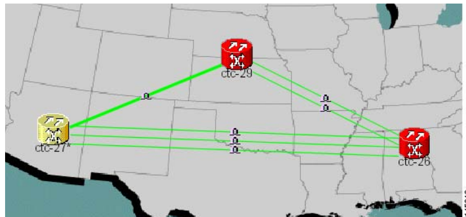
Figure 10-4 Network View with Local Link Consolidation
