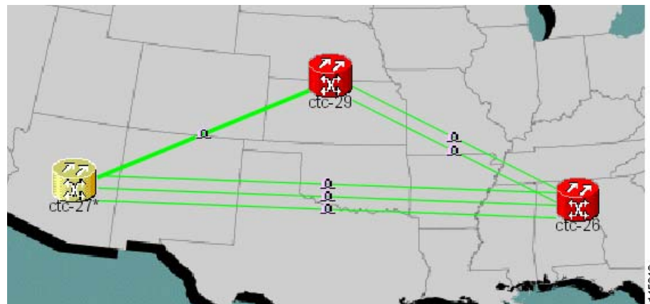
Figure 10-4 Network View with Local Link Consolidation
