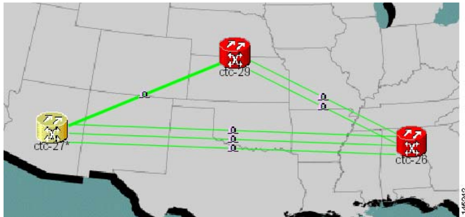
Figure 21-15 Network View with Local Link Consolidation
