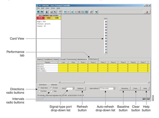
Figure 8-1 Viewing Electrical Card Performance Monitoring Information
