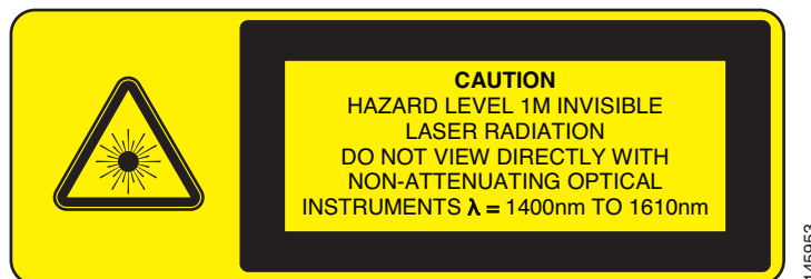
Figure 6-1 Hazard Level Label
