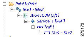
Figure 1-3 Point-to-Point Traffic Demand in the Project Explorer
