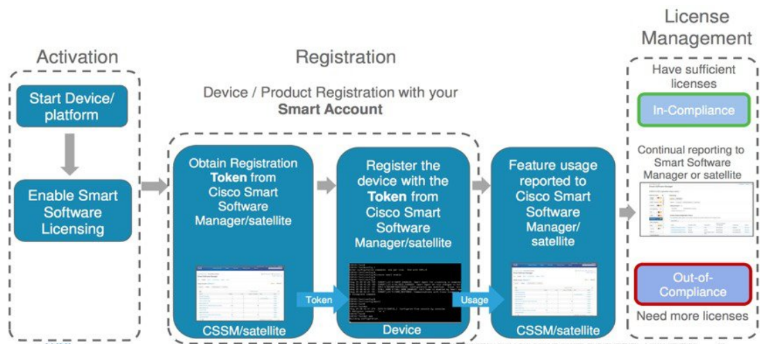
Figure 11: Smart Licensing Work Flow
