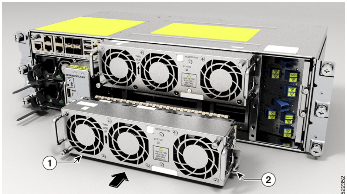
Figure 11: Inserting a Fan Tray
