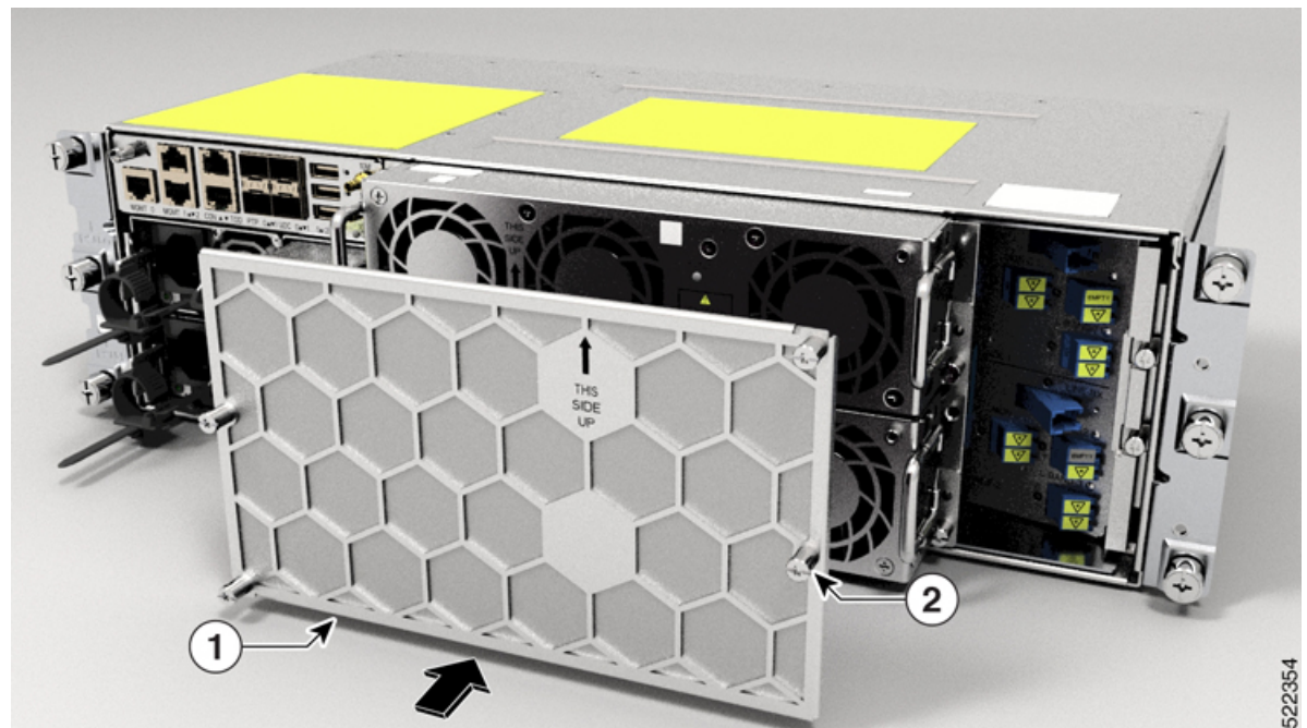
Figure 12: Installing the Fan Filter
