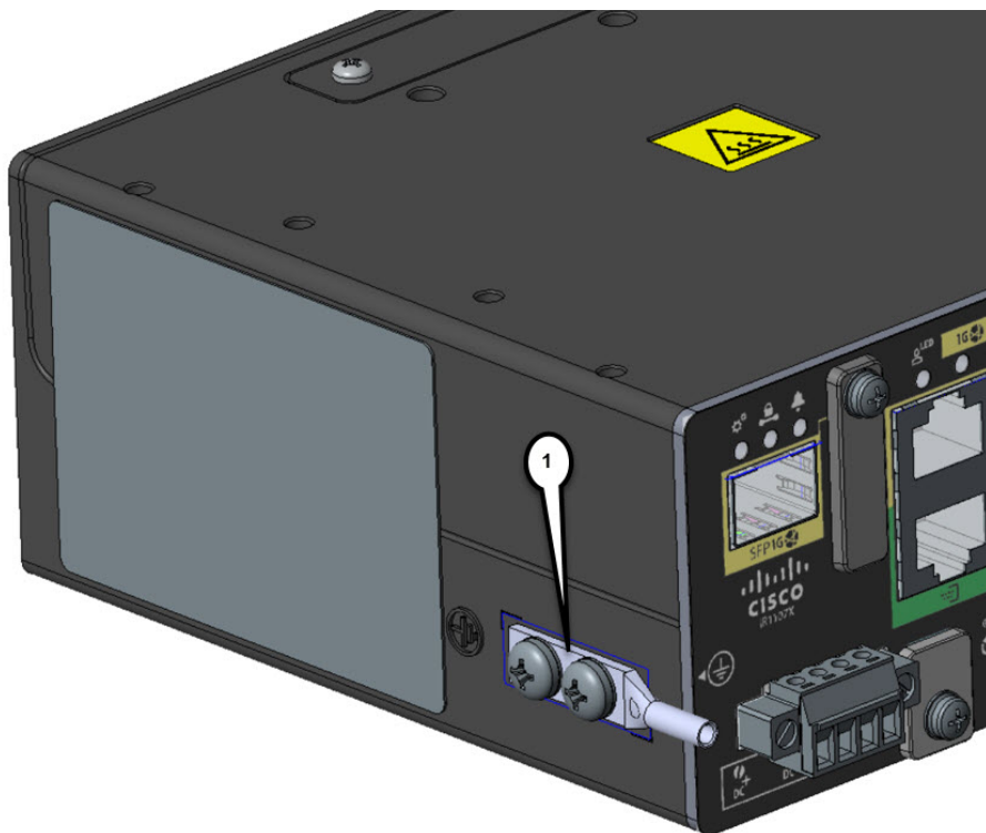
Figure 19: Chassis Ground Connection Points
