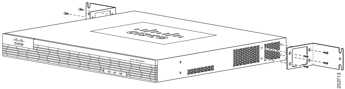
Figure 4-6 Bracket Installation for Back Mounting the Cisco 1905 and Cisco 1921 ISRs
