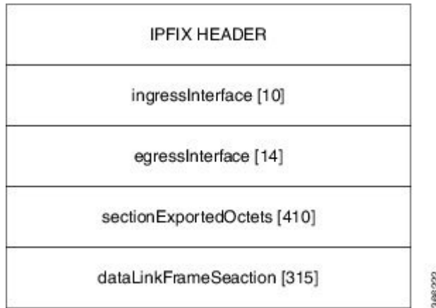
Figure 2: IPFIX 315 Export Packet Format
