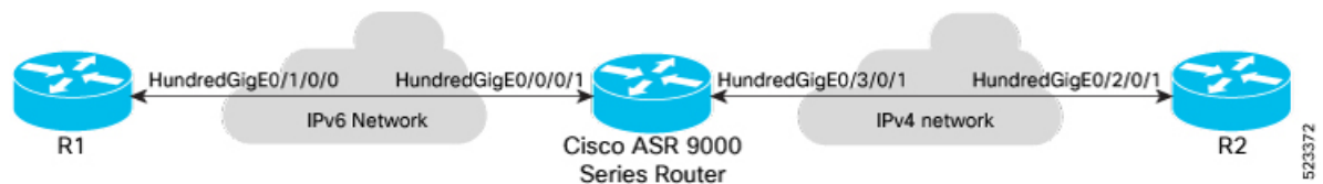
Figure 3: MAP-T L4 packets (Non-TCP/UDP/ICMP) and ICMP Error Messages Handling Topology
