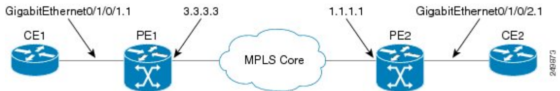
Figure 38: VPLS with BGP autodiscovery and BGP signaling
