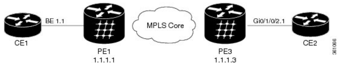
Figure 53: PBB-EVPN on Single Homed Device/Single Homed Network
