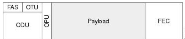
Figure 43: OTN Optical Channel Structure
