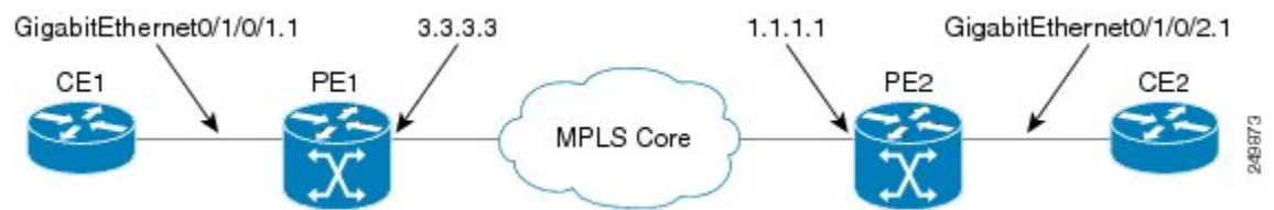
Figure 35: VPLS with BGP autodiscovery and BGP signaling
