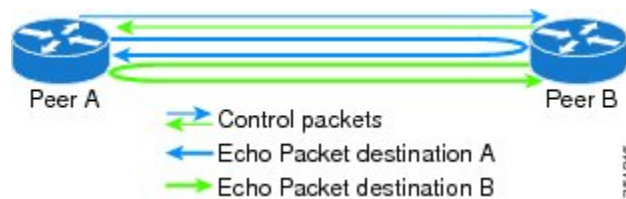
Figure 18: BFD Asynchronous Mode With Echo Packets
