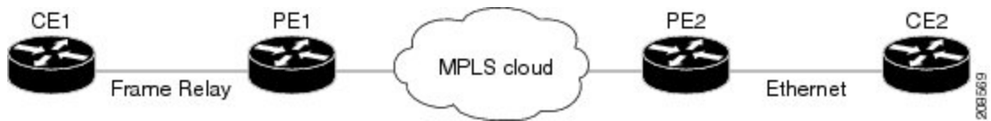
Figure 9: IP Interworking Over MPLS
