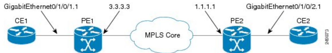
Figure 37: VPLS with BGP autodiscovery and BGP signaling
