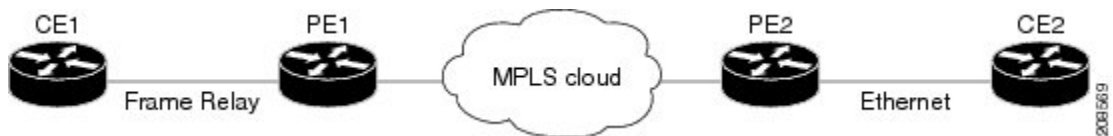
Figure 9: IP Interworking Over MPLS
